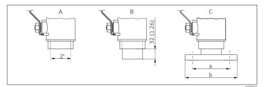
■ 11 Dimensions of process connections in mm (in)
