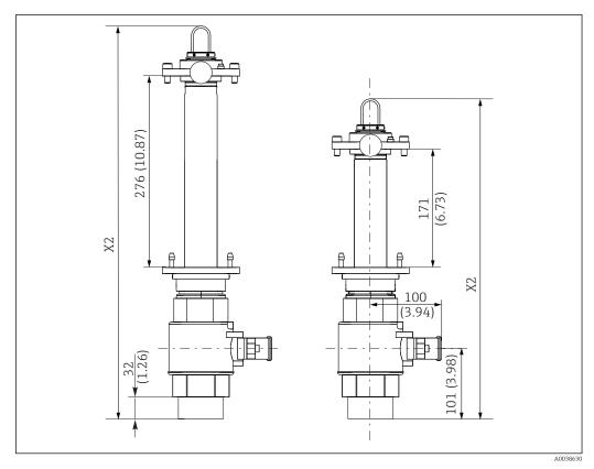
Assembly with G2 thread and weld-in adapter in service position (long and short stroke)
